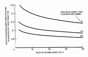
Figure 3.--Ratio of windspeed within (and below) forest canopy to windspeed 20 ft above canopy top.
